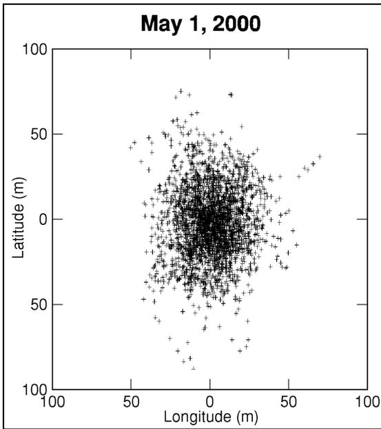
Figure 1: Positional scatter of single-station readings over 24 hours on May 1, 2000 (selective availability on)
