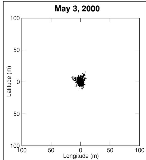
Figure 2: Positional scatter of single-station readings over 24 hours on May 3, 2000 (selective availability off)
