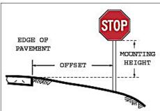
Figure 1. Mounting Height and Support Offset
