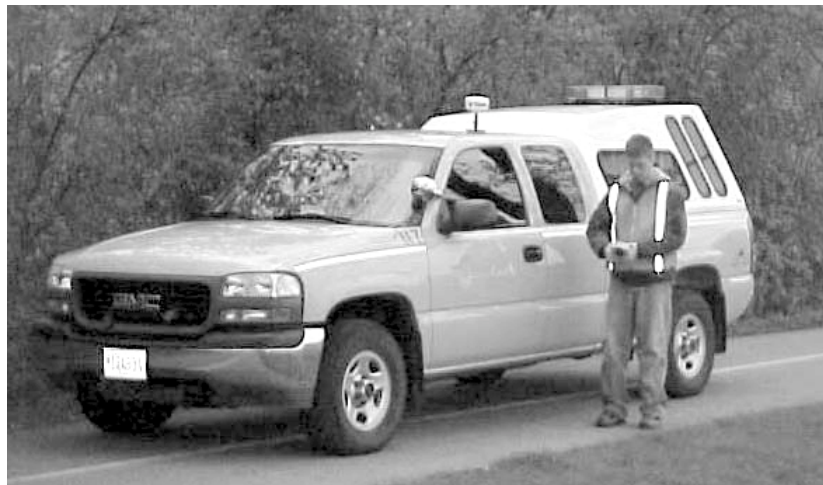
Figure 1. Ryan Williams, GIS Analyst with the Lake County Division of Transportation, stands next to the vehicle used to do GPS mapping of bicycle trails. Note the roof-mounted GPS receiver.
