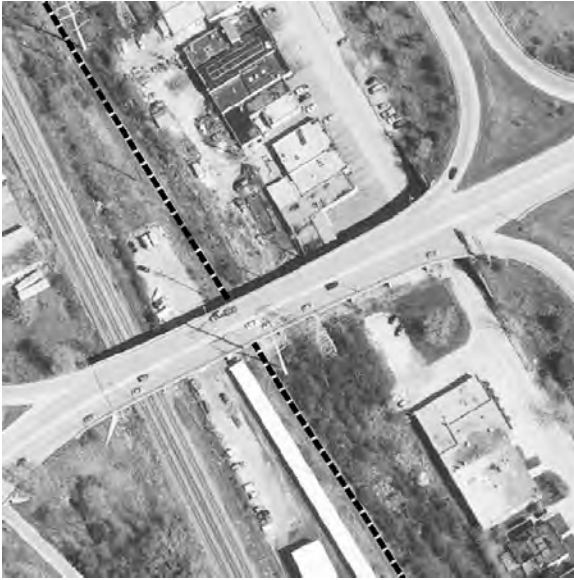
Figure 2. Bicycle trail line theme developed by field GPS data gathering is shown superimposed on a digital orthophoto at a scale of 1" = 100'.
