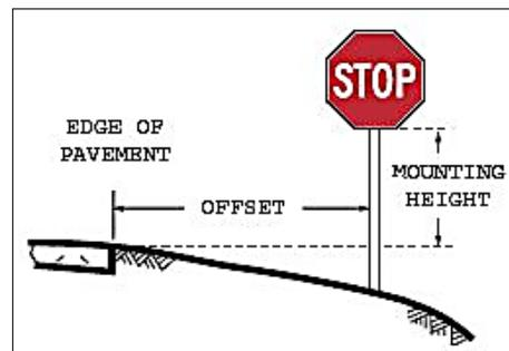
Figure 1. Mounting Height and Support Offset
